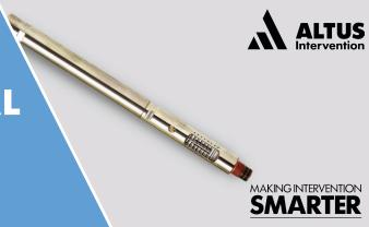
The Fluid Density Inertial (FDI) tool uses the inertial response characteristics of a vibrating tuning fork to determine the density of the wellbore fluid mixture. The FDI tool is a non-radioactive method of determining density that is unaffected by well deviation.
