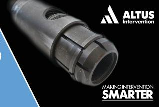
The **PrecisionGS** is used in combination with the **PrecisionStroker** to install completion components eliminating the need for jarring. It consists of a standard GS tool and a release sleeve arrangement that replaces the GS tool shear pin.
